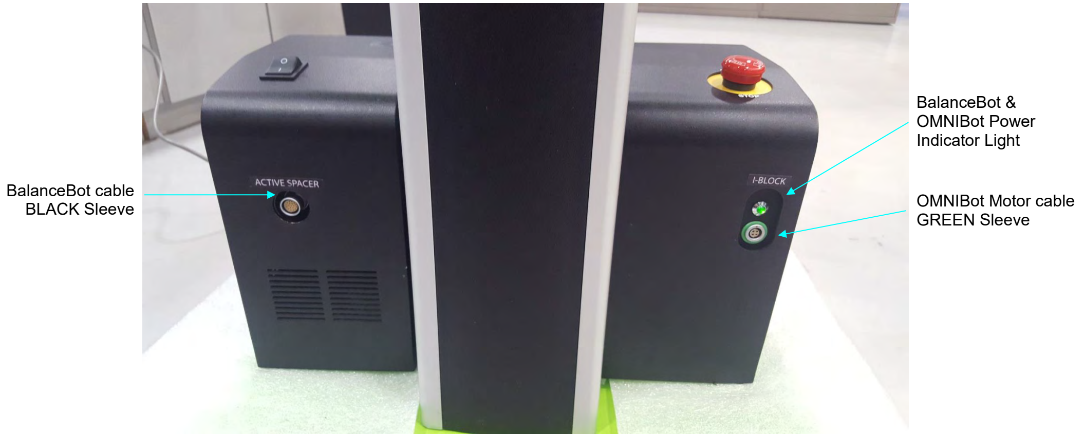
Enclosure Box connections – Front View
