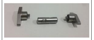
Right Angle Clamp (Part# 1248-0041) has three (3) components. It must be disassembled by unscrewing both locking screws from the post completely. They must be cleaned and sterilised separately,
