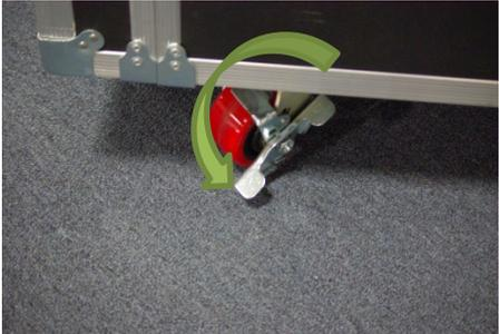
A close-up photograph of a red wheel brake on a metal frame. A green curved arrow indicates the direction to push the brake down to engage it.             |
