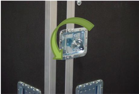
A close-up photograph of a metal latch on a metal frame. A green curved arrow indicates the direction to rotate the latch counter-clockwise to unlock it. |
