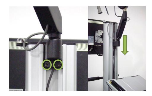
Reinstall small channel cover number 4 above camera arm. Small channel cover 3 can be placed in the storage drawer.
