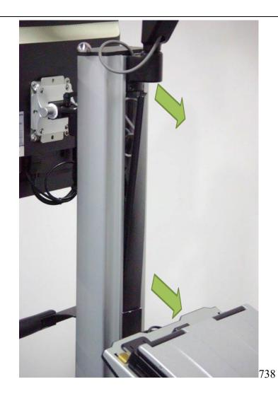
Loosen 2X screws in camera arm and slide arm downward until the top of the camera bracket is slightly below the top of the mast.
