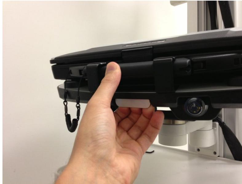
d. If you are leaving the computer unattended at any time, secure it to the Docking Station with the supplied key.
