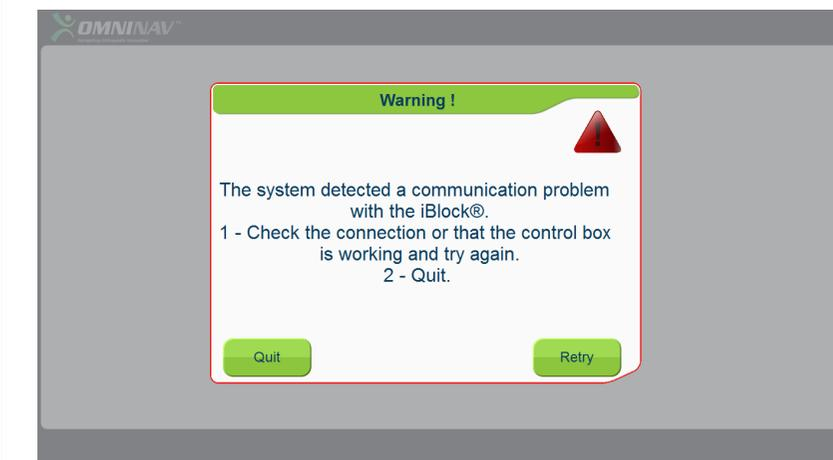
Verify that the Enclosure Box is correctly connected to the Laptop Docking Station at the OMNIBot connection level (USB).
