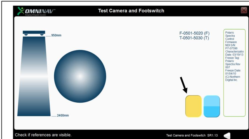
Check that the yellow pedal is functioning correctly by pressing it with your foot. The yellow foot switch icon on the screen will be highlighted.
