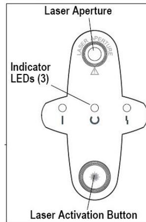
**Laser activation Button:** Press the button to activate the laser. The laser will only remain lit while this button is pressed.
