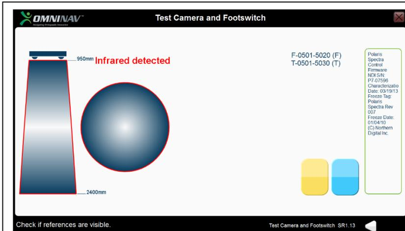
The following screen indicates infrared light interference with the camera (OR lights, presence in front of the camera). The references cannot be tracked.
