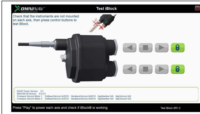
The motor control buttons are not accessible when the axes are unlocked.
