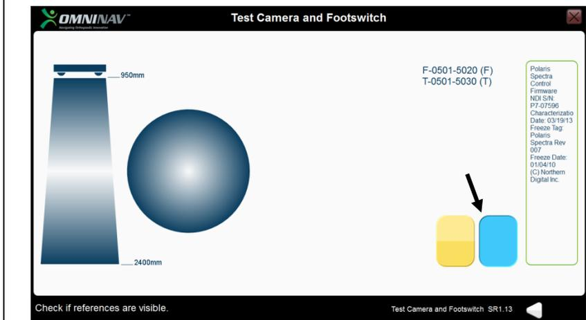
Check that the blue pedal is functioning correctly by pressing it with your foot. The blue foot switch icon on the screen will be highlighted.
