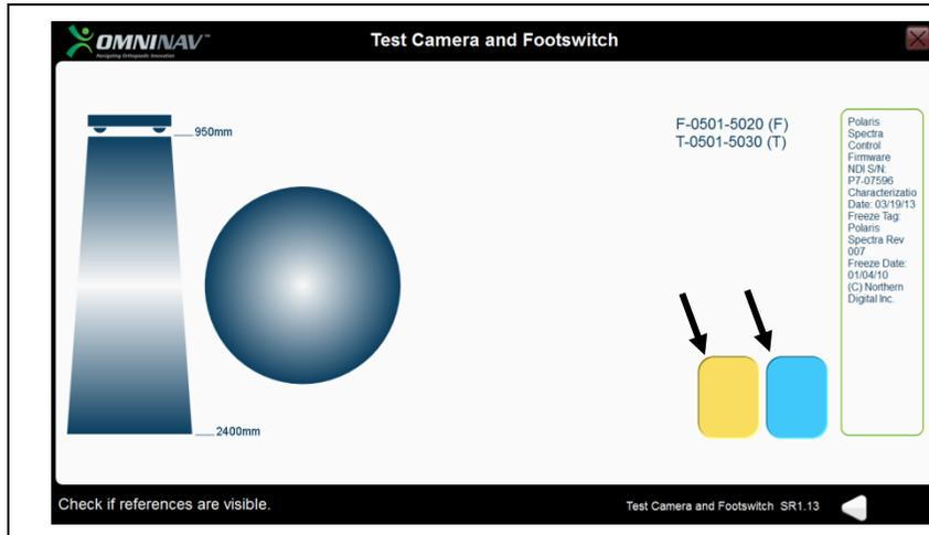
Check that the black button is functioning correctly by pressing it with your foot. Both the blue and yellow foot switch icons on the screen will be highlighted.
