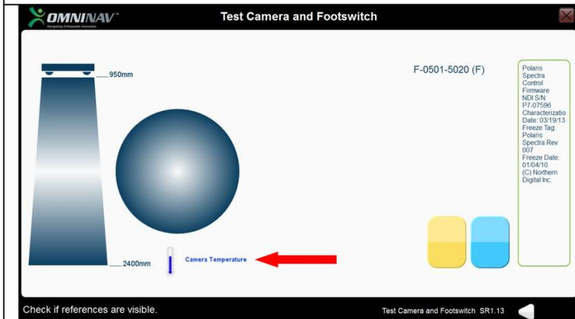
The following screen indicates that the camera warm up phase is not completed yet (2min). The references can still be tracked but accuracy of the tracking can be affected.
