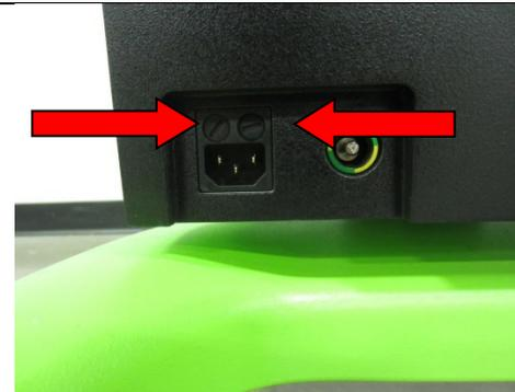
Replace both fuses with new ones and replace compartment.
